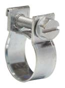
These mini clips, also known as nut & bolt clips, are ideal for small bore hoses with relatively low pressures, where little clamping force is required. Used in low pressure applications such as fuel lines.
